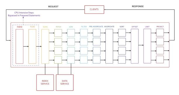
The N1QL Optimizer analyzes the query and available access path options for each keyspace (bucket) in the query. For each query block, the planner needs to first select the access path for each bucket, determine the both join order and type.
